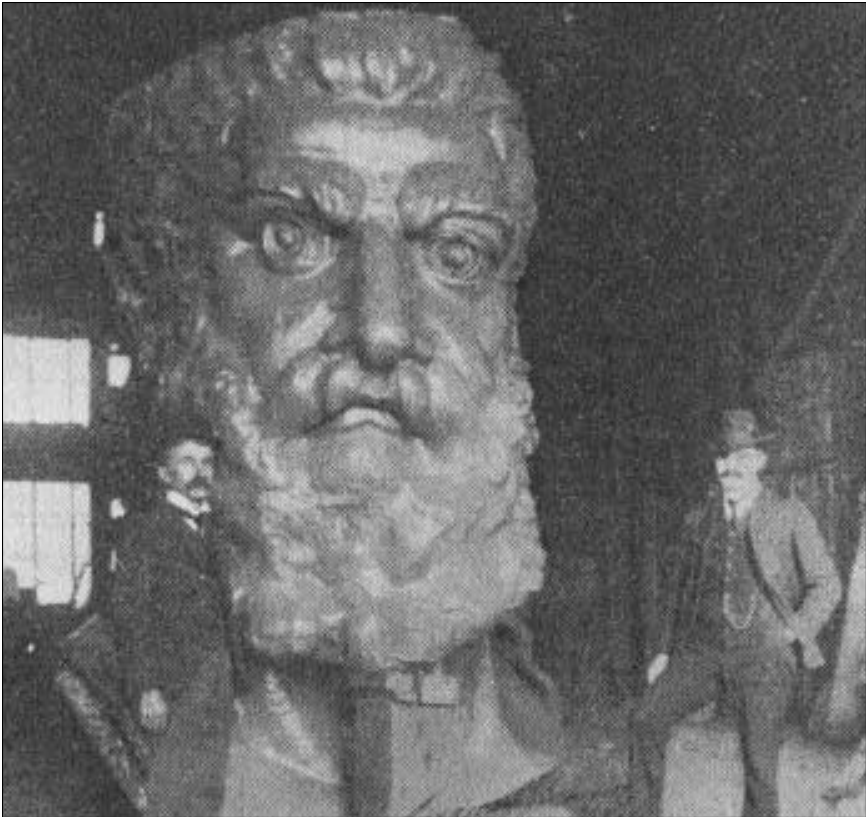
This photograph published in a 1905 American Machinist article shows the completed casting of Vulcan's head, which weighed approximately 15,000 lbs. Library of Congress.
